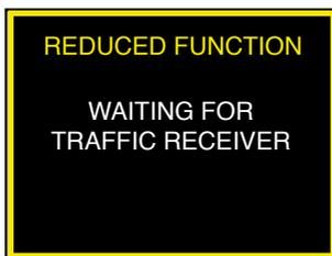
Figure 7.1.: ATD-57 not receiving data from a traffic system
