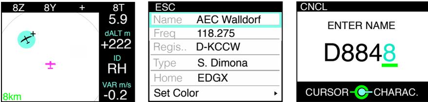
Figure 1.3.: Main radar page, menu, text input page. Inner knob always controls the cyan-colored elements, outer knob the green-colored elements.
