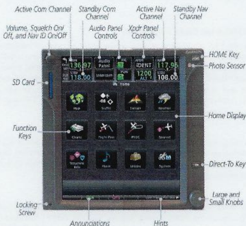
Figure 1 - GTN 750 Control and Display Layout
